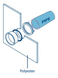
Orientative guide for nozzles installation.
